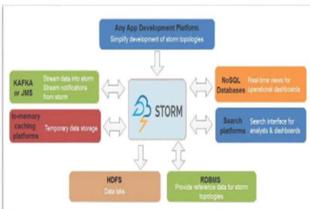
Figure 2. Apache Storm Architecture [20]
